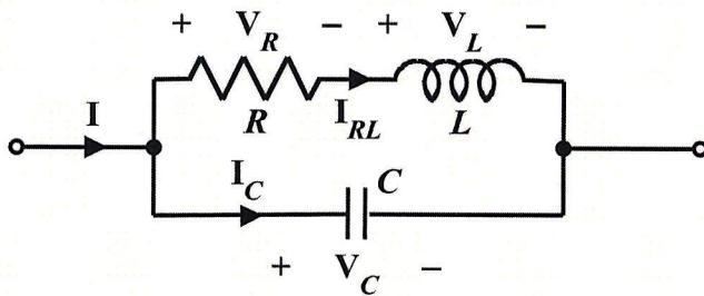
If  $R = 20\Omega$ ,  $L = 5\text{mH}$ , and  $C = 0.5\mu\text{F}$ :
